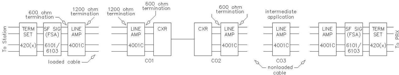
**FIGURE 5.** Typical 4Wire DX Signaling Application Using 104001C Line Amplifiers.
