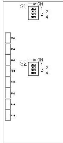
**4.07** To adjust the levels at the splitter output ports, first set S2-3 and S2-4 as described in paragraph 4.06 and then request that 1004hz test tone be sent from the distant end at the level specified on the CLR. With a 600-ohm terminated voltmeter connected to the split out 1 jack, adjust the split out level 1 control to the level required by the modem connected to port 1. Repeat this procedure for the remaining split out ports.
